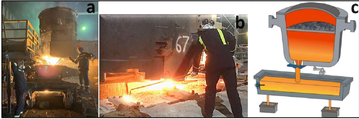
Figure 4. Standard temperature measurement practice (a & b), CasTemp measurement practice (c).
