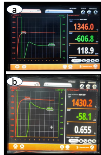
Figure 2. Example of Online Sulfur Measurement Screen (a), Example of Online Silica Measurement Screen (b).
