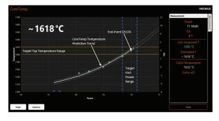
Single measurements are to check if the bath is molten to begin the refinement phases of the process.
